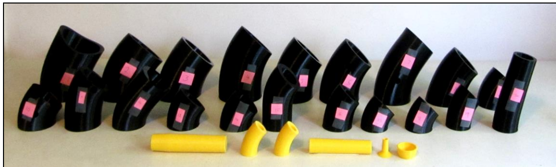
Figure 6: 3D printed parts for the "Anon" serpent prior to assembly
