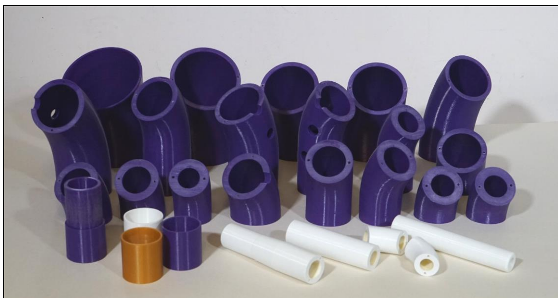
Figure 7: 3D printed parts for the "Dittes" prototype (v3 shown) serpent prior to assembly. v5 parts are similar but not identical.
